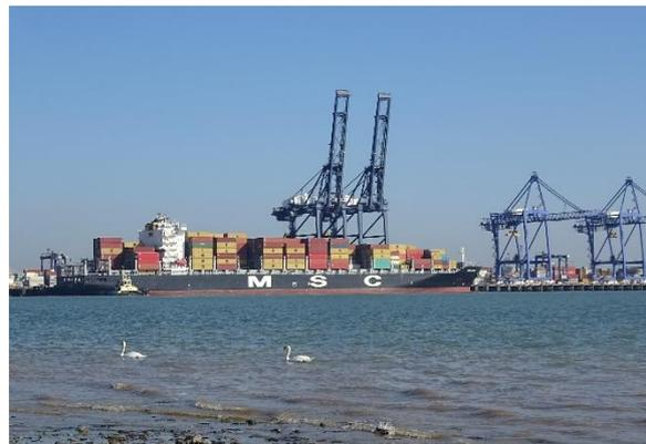
Arriving at Felixstowe, the MSC Vigo is assisted by a single tug to berth alongside the quay. The two ship-to-shore gantry cranes on the quay have their booms raised to prevent a collision with the ship's superstructure as she is manoeuvred into position on the berth. Once the mooring ropes are secured and the gangplank lowered, any final port procedures have to be completed before operations can begin.
